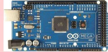
Gambar 2.2 Arduino Mega 2560
