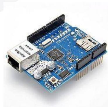
Gambar 2.4 Ethernet Shield
