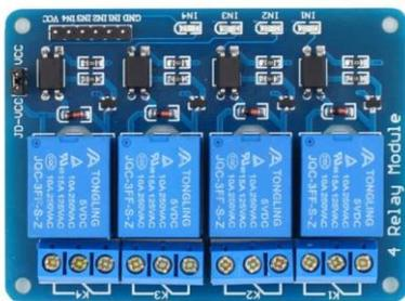
Gambar 2.4 Relay 4 channel
