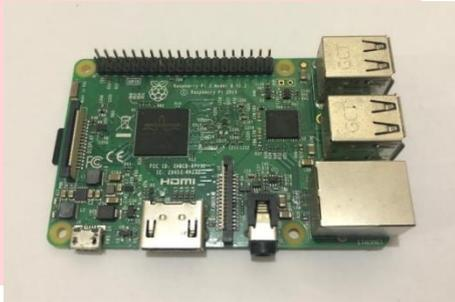
Gambar 2. 1 Raspberry Pi 3 Model B
