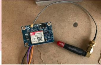
Gambar 2. 5 Modul GSM800L V2
