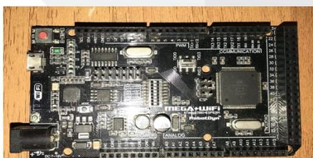
Gambar 2. 2 Arduino MEGA 2560
