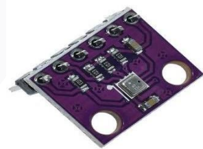
Gambar 2.4 Sensor Kelembaban BME280
