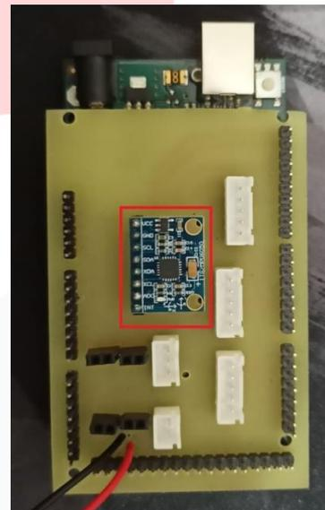
GAMBAR 9 (POSISI SENSOR IMU MPU6050)
