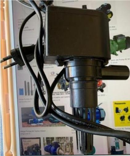
**Gambar 1 Pompa Air**
