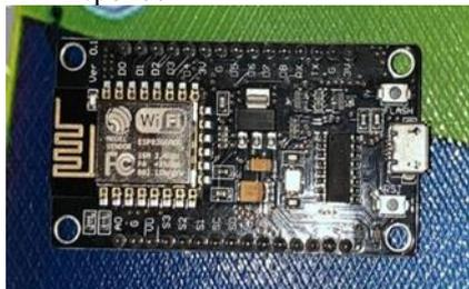
**Gambar 2 NodeMCU**
