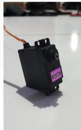
Gambar 2 – 3 Motor Servo MG996R
