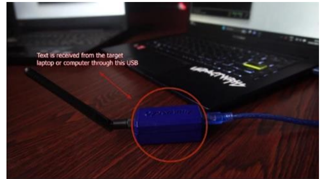
GAMBAR 4.6 Penerima USB keylogger
