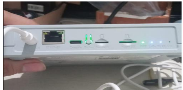
GAMBAR 7 Interface Gateway Sensecap LoRAWAN
