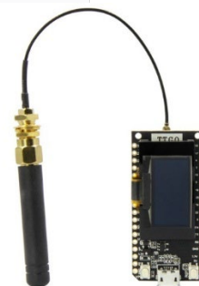
GAMBAR 1 TTGO LORA ESP32 [6]
