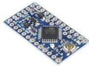
Gambar 9 Arduino Pro Mini
