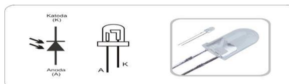
Gambar 2.3 Photodioda
