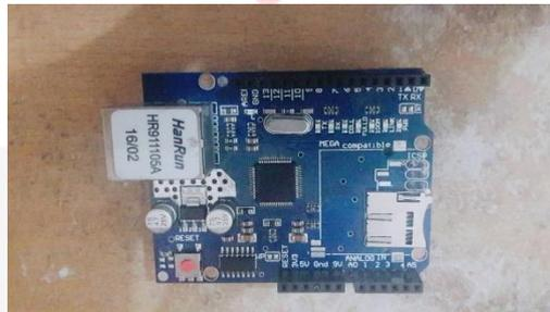
Gambar 4 Arduino Ethernet Shield
