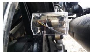
Gambar 4.2 Casing pelindung sensor tampak belakang.
