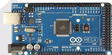
Gambar 2.2 Arduino Mega
