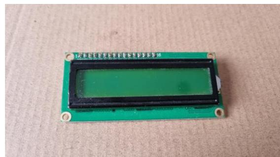
Gambar 2.7 LCD 16X2
