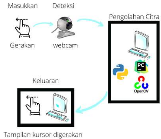
GAMBAR 3. 1 BLOK DIAGRAM PERANCANGAN VIRTUAL MOUSE
