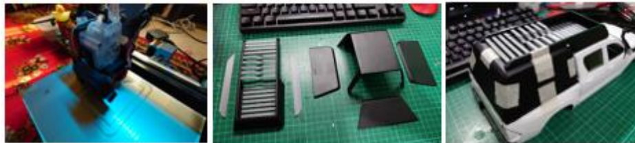
Gambar 4.14 Proses 3D printing dan body part hasil 3D printing (Sumber : Dokumentasi Pribadi)
