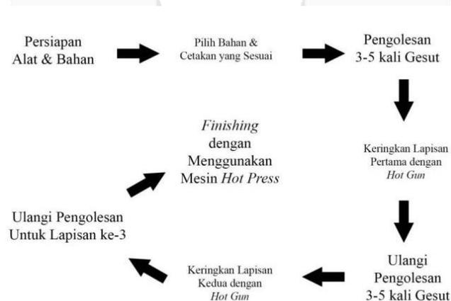
Gambar 3. Skema Proses *Screen Printing* Industrial
