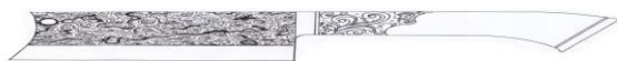
Fig. 18. Design of pamor knife Mrutu Sewu . Specification: Kind of knife: cut, split (with thick and wide knife shape, so strong and sturdy knife, more useful for cutting and splitting hard objects). (Design by Suyono, 2016)
