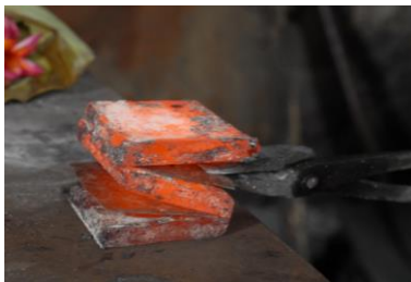
Figure 24. The filling of nickel in wrought iron as a pamor material.
