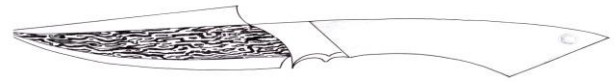
Figure 21. Design of pamor knife Ngulit Semangka . Specification: Type of knife: slice, puncture (The sharpness of this knife is in the lower side, top and in the edge, so it is more suitable for piercing forward and sharp on the curved bottom side more suitable for slicing or cutting) (Design by Suyono, 2016)
