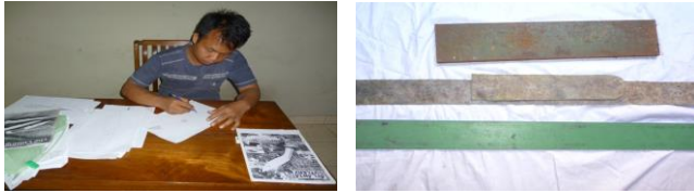
Figure 22, Suyono is making work drawings to make prototype works. Figure 23, the main ingredient used to make a pamor knife which includes: Wrought iron weighing 15 kg, Steel 01 weighing 3 kg, Nickel weighing 500 grams, and wood.
