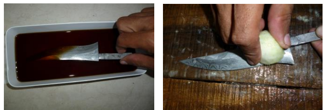
Figure 26 (left), the process of forming the pattern of pamor Nguntu Walang , the process is using drip or chisels ( betel ) which is unsharpening by placing on drip at the end of the blade which will imprint according to the wound produced in the drip or that chisels ( betel ). Figure 27 (right), a knife material in gedeq to create a pattern of pamor Nguntu Walang . Figure 28 (bottom), the formation of knife detail with grinding tool machine.
