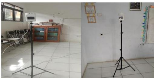
Gambar 2. Alat Ukur Suhu Tubuh Berbasis Sensor Infrared
