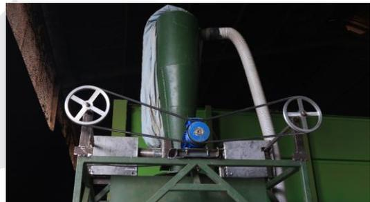
Gambar 8 Prototype Alat Bantu Dust Collector
