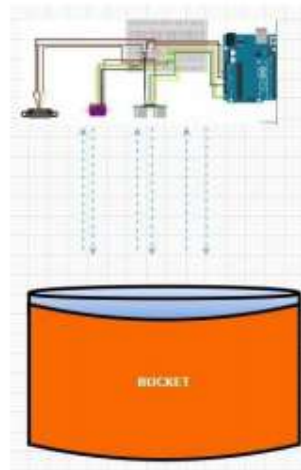
Figure 3.3 Illustration of how Arduino measurement the distance
