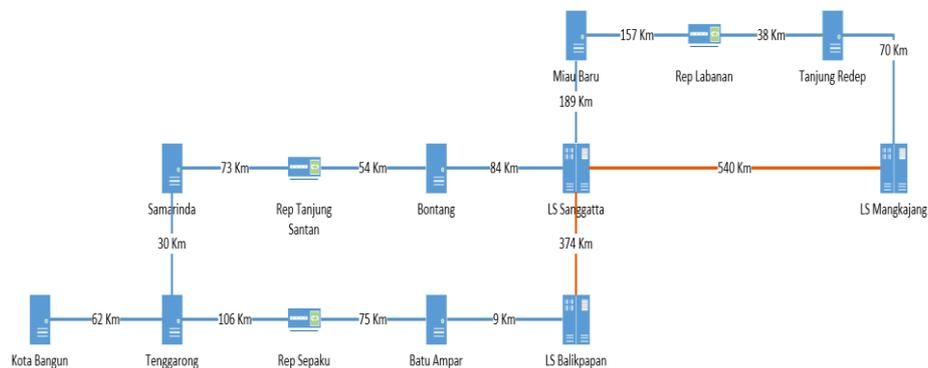
Fig. 2. Terrestrial Network Topology and SCCS Network.
