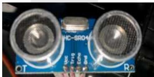
Gambar 1. Sensor ultrasonik
