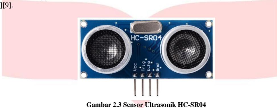
Gambar 2.3 Sensor Ultrasonik HC-SR04
