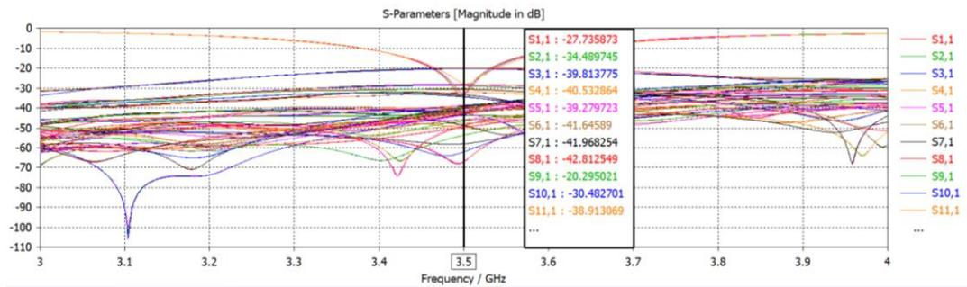
Gambar 7. Grafik Mutual Coupling Antena MIMO 2x8
