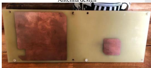
FIGURE 4 Front view fabricated antenna
