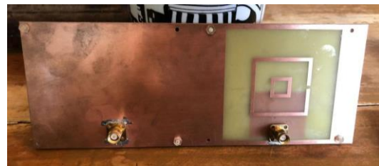
FIGURE 5 Rear view fabricated antenna
