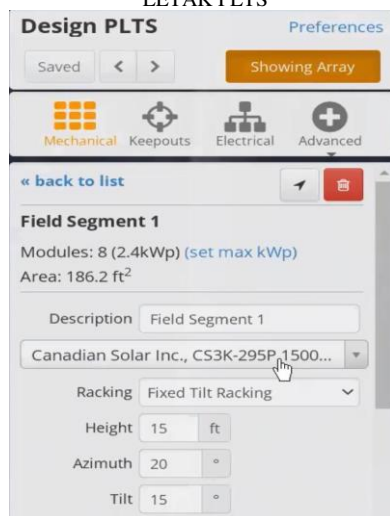
GAMBAR 9 PANEL SURYA, TILT, DAN AZIMUTH
