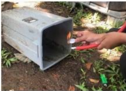
GAMBAR 3 Uji Bakar Gas Metana
