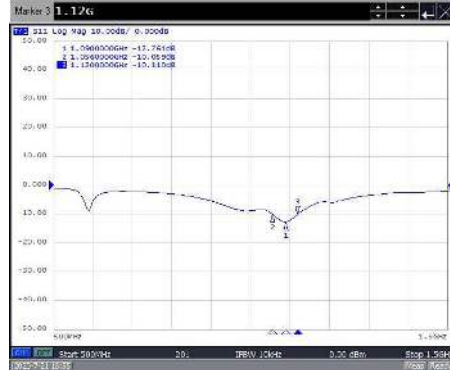
Gambar 26 Hasil Pengujian Return Loss ADS-B
