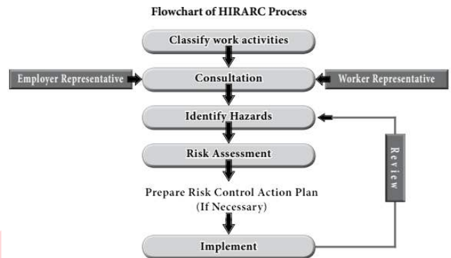
FIGURE 2. Flowchart of HIRARC Process (Source: DOSH, 2008)
