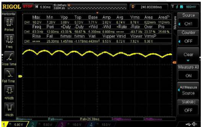
Gambar 4.3 Hasil pengujian Three Phase Rectifier tanpa kapasitor
