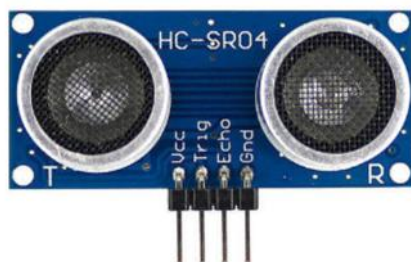
GAMBAR 2.1 Sensor Ultrasonik HC-SR04
