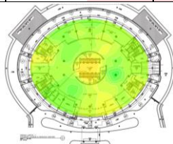
FIGURE 5 1st floor signal strength
