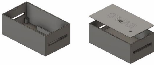
FIGURE 2.3 EVPLC Module Casing Design
