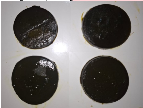
GAMBAR 2 (SCAFFOLDS VARIASI KONSENTRASI GELATIN 2%, 4%, 6%, 8%)
