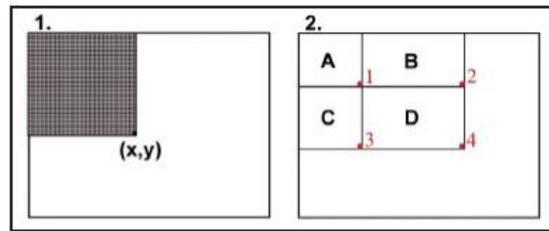
Gambar 2.3 Konsep penghitungan integral image (Source : <http://www.bantronix.com/2011/10/face-recognition.html>)
