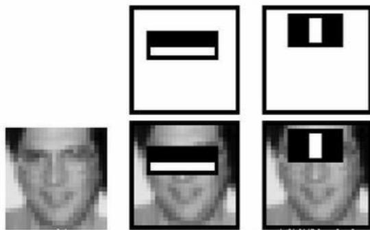
Gambar 2.5 Contoh pencarian dengan haar-like feature (Source : [http://docs.opencv.org/trunk/doc/py\\_tutorials/py\\_objdetect/py\\_face\\_detection/py\\_face\\_detection.html](http://docs.opencv.org/trunk/doc/py_tutorials/py_objdetect/py_face_detection/py_face_detection.html))
