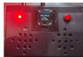
GAMBAR 11 HARDWARE NODE RECEIVER TAMPAK ATAS
