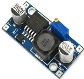
GAMBAR 15 Step Down LM2596
