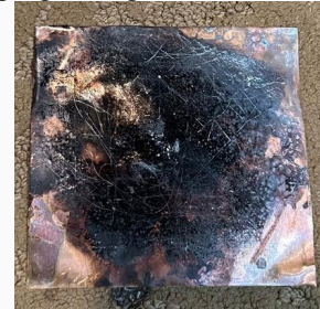
GAMBAR 8 Efek Korosif NaOH
