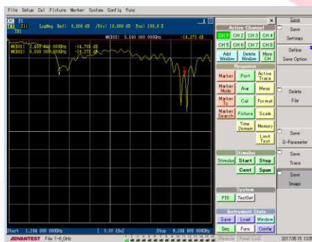
Gambar 4. 1 Pengukuran Return Loss
