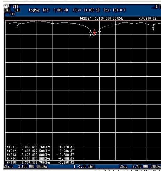
Gambar 4.4 Return loss realisasi
