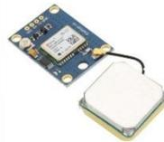
Gambar 2.1 GPS module UBLOX NEO 6MV2[3]
