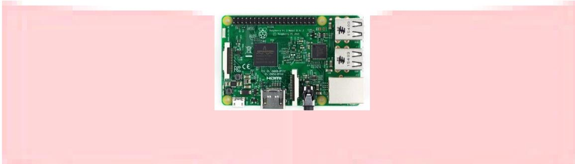
Gambar 2.2 Raspberry pi 3 model B[3]
