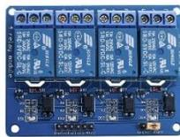
Gambar 2.3 Relay 4 channel[15]
