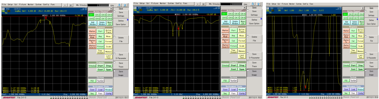
Gambar 7. Insertion Loss Hasil Realisasi (A) Return Loss Hasil Realisasi (B) VSWR Hasil Realisasi (C)
