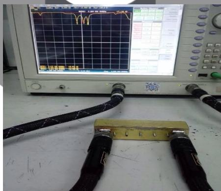
Gambar 6. Realisasi Bandpass Filter *Comblaine Cavity*
