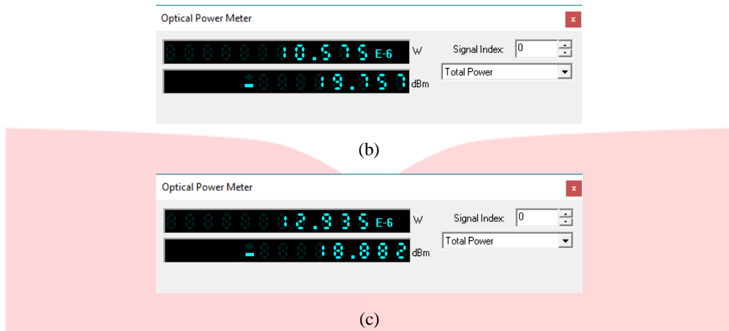
Gambar 4.2 Hasil power received terburuk tiap kecamatan (a) Kec. Loksado (b) Kec. Kandangan (c) Kec. Kalumpang sisi upstream
