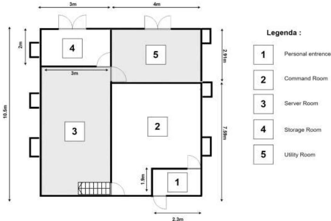
Gambar 4 Denah Usulan Ruangan Data Center
